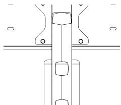
Running down the back of the mast is the cable mangement. Designed so that leads and wiring can be neatly and efficiently tucked away.
