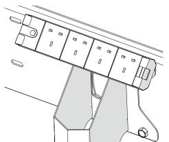
4-way UK power socket included as standard. Located at the top of the mast (behind the screen), users can utilise the power and cable management straight away.
