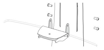
A series of slots run along the front of the Axia's mast allowing users to place the shelf at their optimum height.
