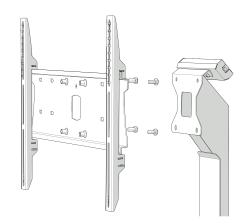
Both Pozimount Universal Mounts or Xactmatch Dedicated Mounts easily fit straight onto the mast of the stand or trolley, giving you the freedom to choose.
