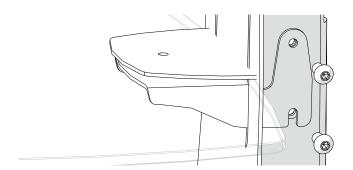
Once the optimal location has been determined, simply screw and tighten into place. Shelves can support up to 20kg.
